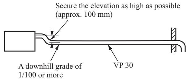
(e) The stiff PVC pipe put indoor side should be heat insulated.
