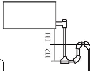
H1=100mm or the static pressure of air sending motor
