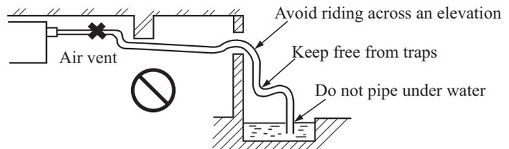
(b) When connecting the drain pipe to unit, pay sufficient attention not to apply excess force to the piping on the unit side. Also, fix the piping at a point as close as possible to the unit.
